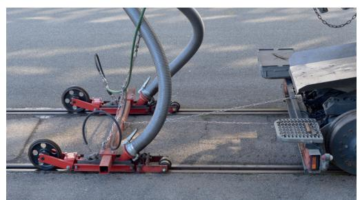
Tunnel cleaning/wet cleaning of arched tunnels, shoulders and lanes (Euroclass 5 low-emission motor with a soot particle filter)
